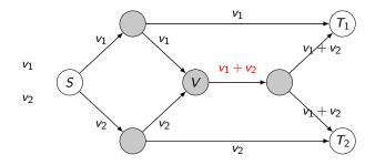
$\min$ -cut $(S, T_1) = \min$ -cut $(S, T_2) = 2 \implies \mu(\mathcal{N}) = 2.$
