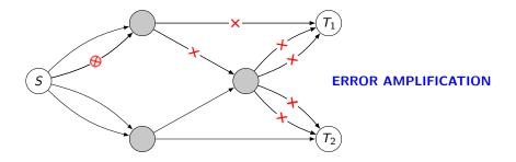
Natural solution: design the node operations carefully (decoding at intermediate nodes).
