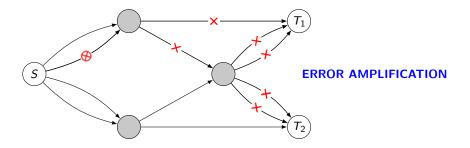
**Natural solution:** design the node operations carefully (decoding at intermediate nodes). **Other solution:** use rank-metric codes.
